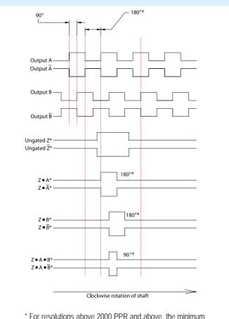
$<sup>^*</sup>$  For resolutions above 2000 PPR and above, the minimum edge separation can only be guarenteed to  $50^{\circ\,\text{e}}$
