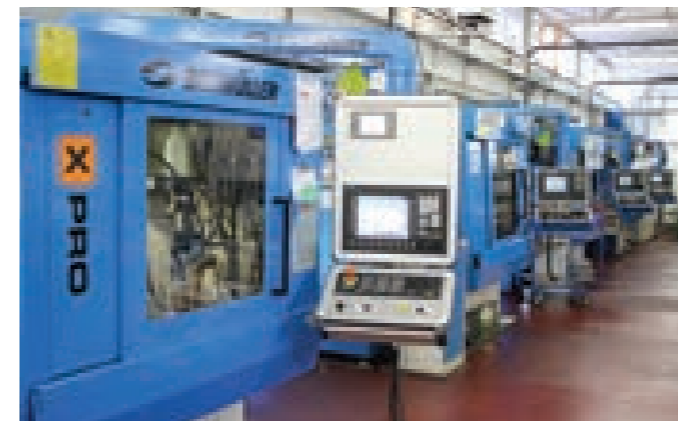
After heat treat, all critical dimensions and raceway geometries are precisely machined to the micron ( \mu ) in our grinding department!
